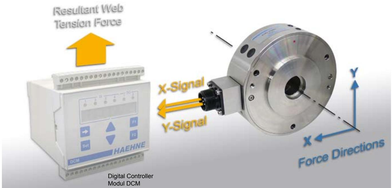
The Dual Axis Web Tension Sensor XYR measures simultaneously in the X-and Y-direction. Traditional radial force sensors measure generally only in one preferred direction. Measuring effects in other directions are typically unwanted because generally they result in measuring errors.
